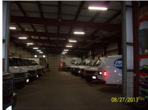
The vans are good candidates for conversions but do face some challenges. The main issue is finding enough space for the CNG tanks used in the conversion. Each van is equipped with a refrigerator unit used to transport goods. Together with the unrefrigerated product, it does not leave a lot of room in
