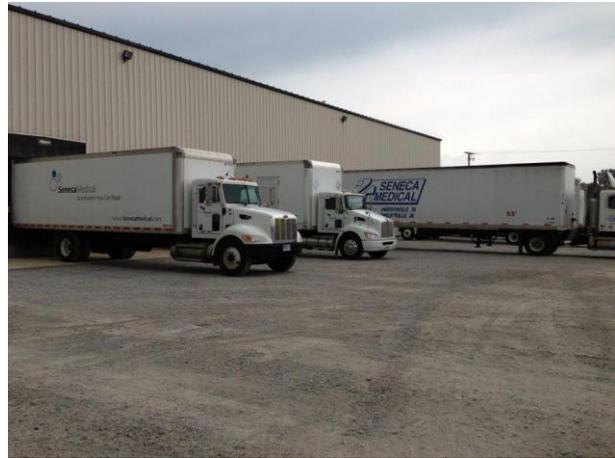
Conversions for these trucks will consist of a dual fuel setup. Straight trucks have more than enough room for the new CNG tanks between the wheels. Capacity of the tanks therefore will only be limited by the necessary amount of CNG needed for each truck's route. The tractors on the other hand do not have the luxury of unlimited room, and therefore will have to have a system designed to balance capacity and storage space on a truck by truck basis.
