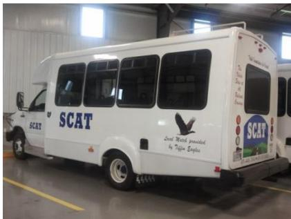
The conversion of a transit van consists of a bi-fuel setup with the CNG tanks mounted under the vehicle. The bi-fuel setup allows the vehicle to be powered by CNG when it is present, and gasoline should the CNG run out.
